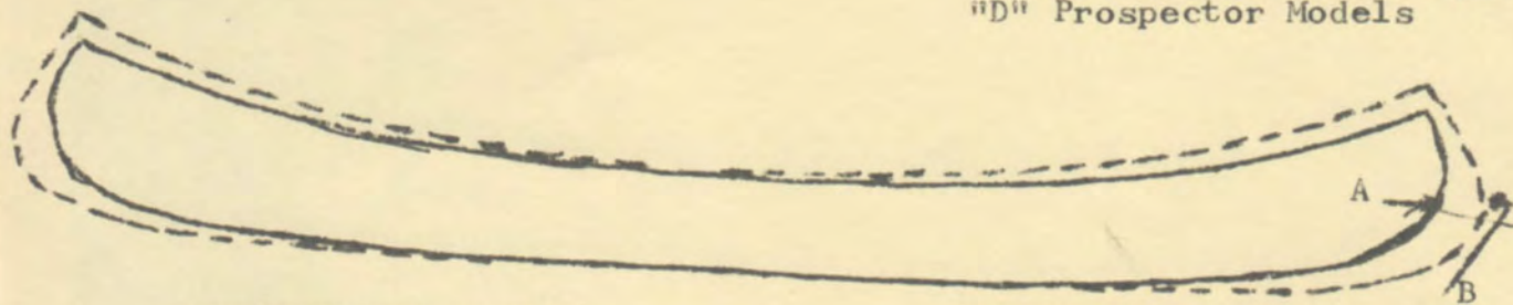
LONGITUDINAL DESIGN SAME BOTH ENDS "A" - Freighter, Pleasure, Prospector, Cruiser & Guide Specials "B" - Ogilvy Models
