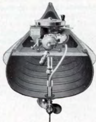
Sectional view of Sponson Canoe with motor installed.
