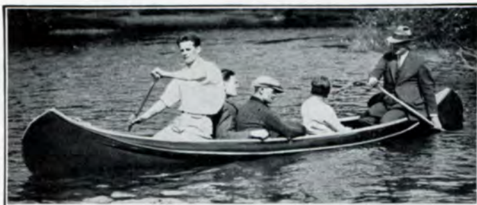
16-foot "Sponson Floatwell" Canoe carrying five persons (800 lbs.) No overload. Note the good freeboard.
