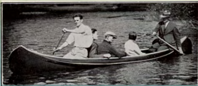
16-foot "Sponson" Canoe carrying five persons (800 lbs.). No overload. Note the good freeboard.
