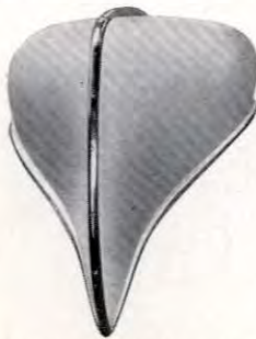
POLISHED BRASS BANG PLATES, PRESSED TO CORRECT FORM, PROTECT STEM.
