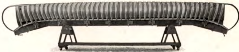
SHOWING HOW RIBS AND STEMS ARE BENT OVER THE FORM
