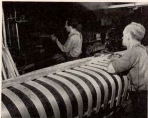
Ribs being steamed on form.
